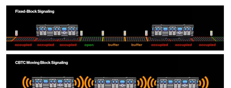
Currently, NYCT's signal system utilizes two types of technology: fixed-block electro-mechanical signaling and modern digital moving-block technology known as Communications-Based Train Control (CBTC), Fixed-block relies on technology that dates to the opening of the subway over 110 years ago. It uses wayside track circuits, signal heads, and train stop arms to enforce speed restrictions and safe distance between trains, as shown in the figure above.
