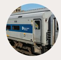
Coaches A railcar that carries passengers; one or more coaches make up a train that is pushed or pulled by a locomotive.
