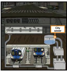
**3.** When sewers are overwhelmed, torrential rainfall events cause water to collect on the street. This stormwater can enter the subway from the street through openings like sidewalk vents and stairs.
