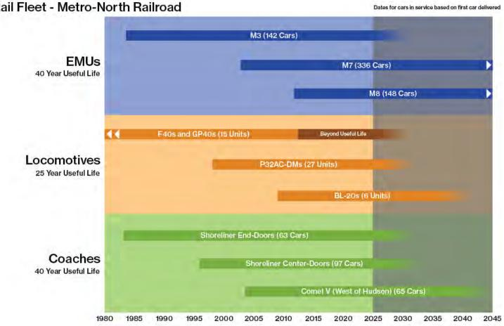
Upgrade the passenger fleet through the continued replacement of the M3 EMUs that have been in service on the Hudson and Harlem lines since the 1980s and are past their useful life. These will be replaced with new M9As that are a next generation railcar equipped with multiple amenities to improve customer experience, including better accessibility,
