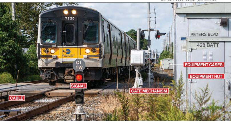
Above, standard LIRR signals system annotated with signals components
