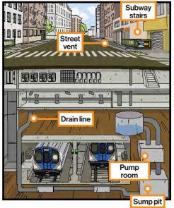
**2.**The subway drainage system connects to the New York City storm sewer system that takes the water to the local wastewater treatment plant.
